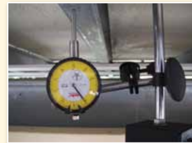
Deflection measurement gauge.
