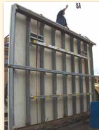
SlenderWall panel outfitted for testing.
